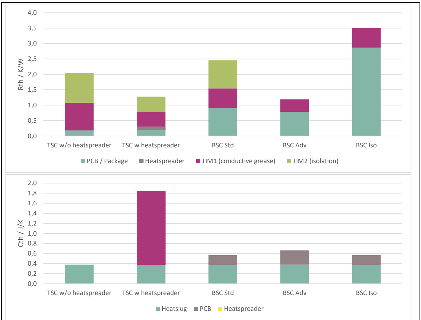
Figure 16 Distribution of the R th and C th contributors for different assembly options
