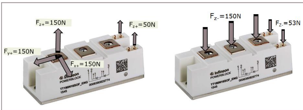
Figure 12.2: Maximum permissible forces during assembly (SB34)
