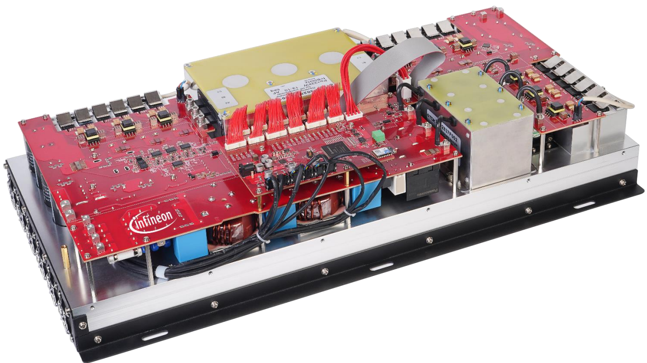
Figure 1 22 kW power converter demonstration system for bidirectional DC EV chargers
