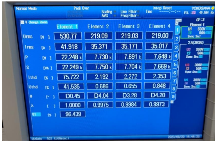
Figure 24 Current, voltage, power, and THD in forward mode at 22 kW
