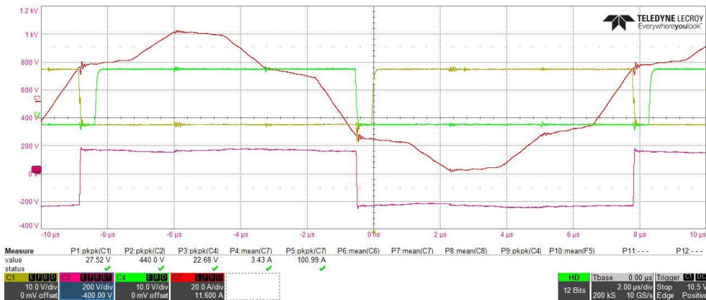
Figure 31 Steady-state waveforms of the current and voltage on the secondary side of the 3-phase DAB converter at P = 22 \text{ kW} , V_{DC} = 530 \text{ V}
