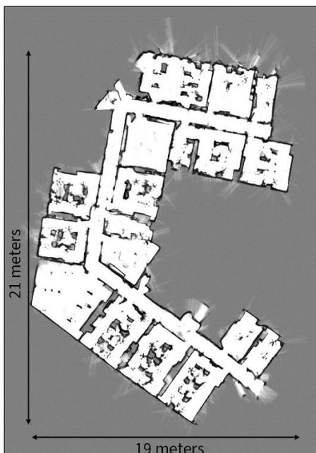
Figure 1: SLAM-generated map using Infineon and pmd's new hToF sensor
